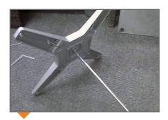
Connect the rod with two screws and washers to the cross.
