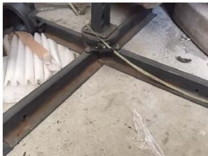
This is a Barca Queen cross base which is starting to show signs of rust. Rust is inevitable; however, it should take years for it to surface. If the umbrella is exposed to the sea air, rust will settle in far quicker than usual. The sea air is extremely corrosive.
