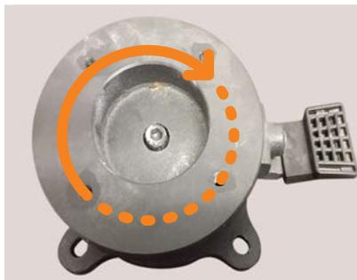
The swivel mechanism runs with ball bearings on the inside, which allows it to turn 360 degrees. If the ball bearings aren't lubricated regularly, the ball bearings will rust and fuse, which prevents the mechanism from swivelling.
